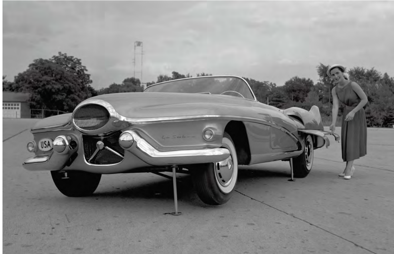
The Le Sabre's built-in hydraulic lifts in action. General Motors LLC
