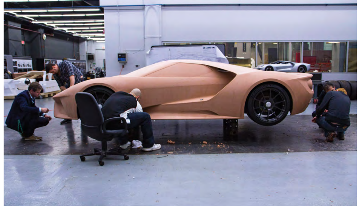
The design team adjusting details on a clay model of the 2017 GT. Ford Motor Company Archives
